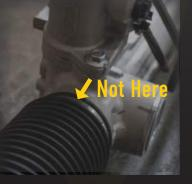
Older rack and pinion assemblies are traditionally equipped with venting tubes that run externally along the length of the part. Internal venting removes the risk of damage and increases the life of the repair while decreasing the likelihood of a warranty failure.
