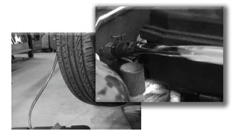
Flushing of the fluid is complete when the fluid exiting through the clear tubing begins to lighten and match the color of the new fluid being added to the reservoir.
